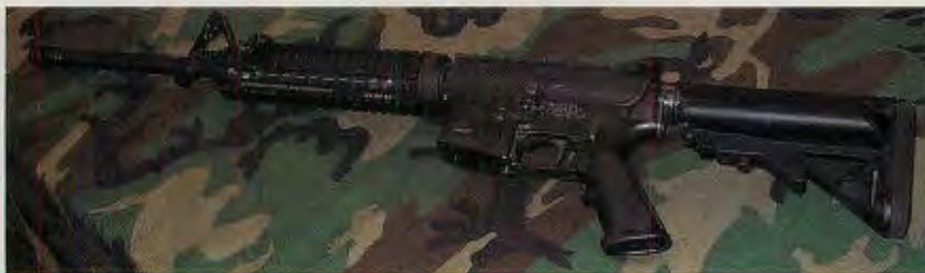
Carbine version of SDM rifle has similar features, but has 18-inch barrel and weighs a pound less – handy for troops in vehicles or helicopters.
